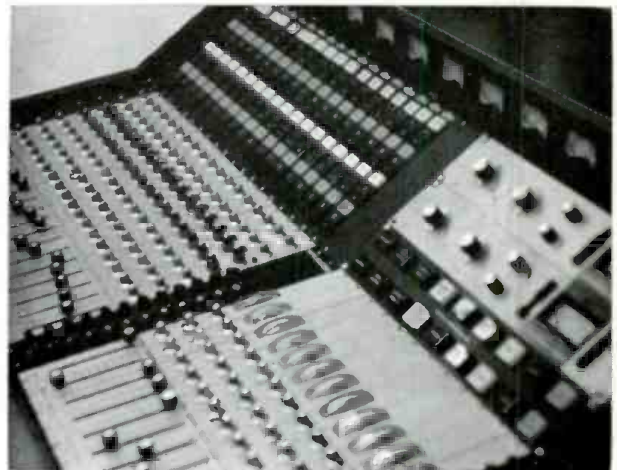
Figure 2. Side view of eighteen input modules (left) and twelve master record/reverb modules (right) surrounded by remote controls and limiters.
